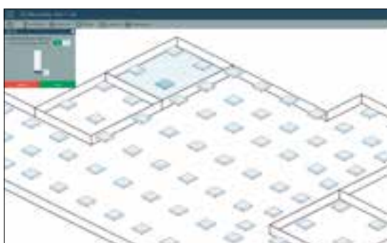
The 3D graphic interface is based on the building's blueprints. Using the drag and drop function, luminaires and components can be assigned to a zone.
