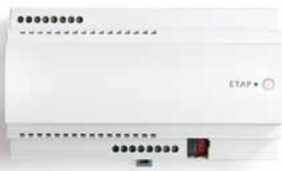
The controller has 4 DALI lines, which can each individually control up to 64 addresses. For large projects, up to five controllers can be linked.
